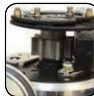
Precision magnetic pickup coil and reluctor.
