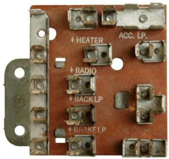
1956 Chevrolet fuse block/fuse panel is an example of a fuse block that was not originally part of the wiring harness but rather a separate component.
