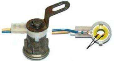
We have been made aware that occasionally customer's experience a problem when installing our reproduction (and even NOS GM) Alarm On/Off Switches. After a new alarm switch is installed, when the door is locked and the key removed, the alarm should be turned-on. But some customers state that while turning the key to lock their car everything works properly (alarm has turned-on) until the final fraction of a turn - when the key is in the position to be removed - that the alarm turns off again.
