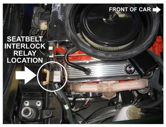
Shown above and below is the Seatbelt Interlock Bypass Relay (with manual bypass button to start) appearing under the hood of a Corvette. The type of bypass relay and its location on other make/model vehicles, may vary.
