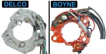
Both the Delco/Guide and Boyne-type turn signal switches were used on early GM cars (except Corvette). These two switches are physically different, and not interchangeable. When replacing your turn signal switch, make certain that you first identify your original switch. The Delco/Guide switch will have either of 3 words molded into the switch: 'Delco Guide', or 'Delco', or 'Guide'. The Boyne switch will have 'BPC' molded into the switch.
