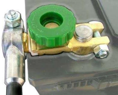
A battery disconnect switch makes it convenient to isolate the battery from any potential draws when the ignition switch is off (like a clock, radio display, glove box light, computer, etc.) and it's much more convenient to turn a knob or move a lever than to keep removing the battery cables from the battery.
