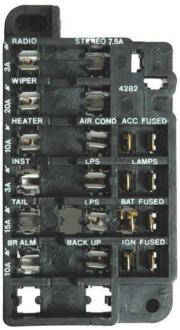
1965 Chevelle fuse block is an example of a fuse block that was originally part of, and integrated into, the wiring harness.
