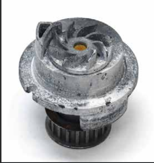
Cooling System Problems: Electrolysis Refer to Page 14
