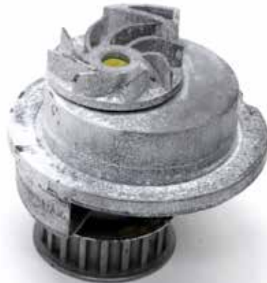
Poor cooling system condition (Electrolysis)
