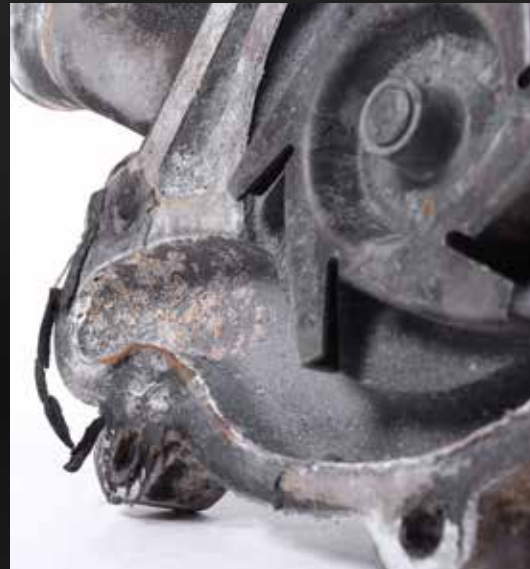
Cooling System Problems: Cavitation Refer to Pages 16-17
