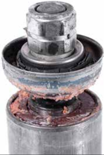
Seal Failure Refer to Page 10
