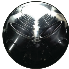
Velocity stacks for better air flow
