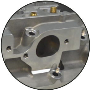
CNC'd ports and combustion chambers
