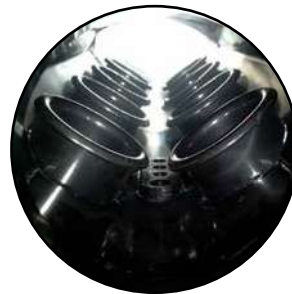
Velocity stacks for better air flow
