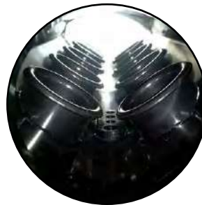
Velocity stacks for better air flow
