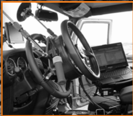
Data acquisition system and robotic steering wheel controller
