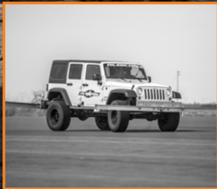
FMVSS 126 test final run, 300 degree right hand turn at 50mph
