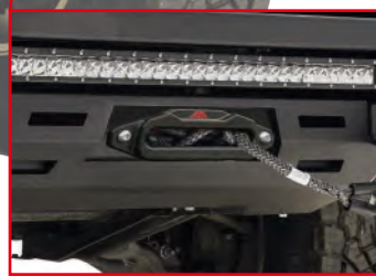
RECESSED WINCH MOUNT WITH INTEGRATED FAIRLEAD PLATE
