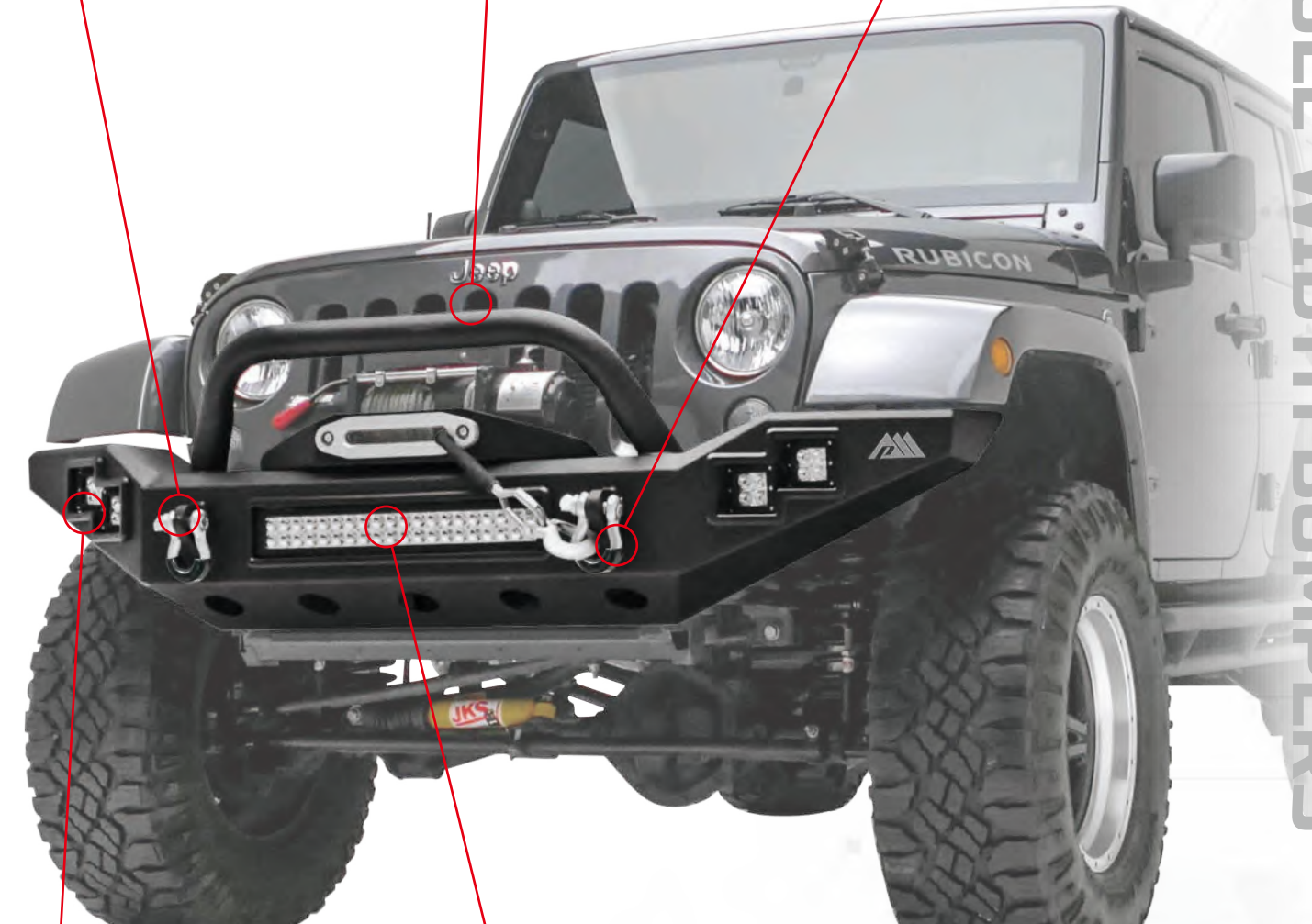
D-RING MOUNTS WELDED INSIDE AND OUT
