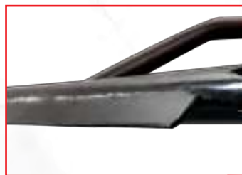
WIND DEFLECTOR ELIMINATES CAB NOISE
