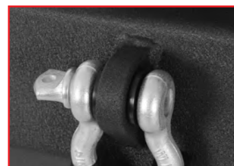
D-RING MOUNTS WELDED INSIDE AND OUT
