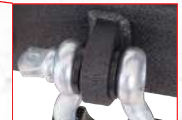
D-RING MOUNTS WELDED INSIDE AND OUT
