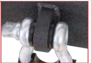
D-RING MOUNTS WELDED INSIDE AND OUT
