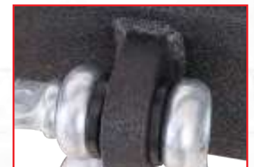
D-RING MOUNTS WELDED INSIDE AND OUTSIDE
