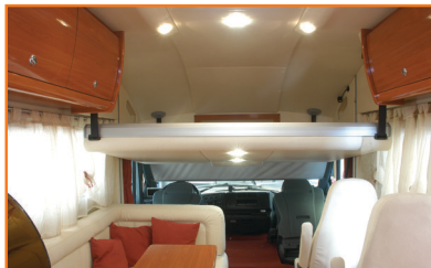
Patented nylon belt system quickly raises and lowers bed
