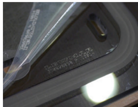
On some Lewmar hatches you may need to peel back the seal slightly to reveal the code.
