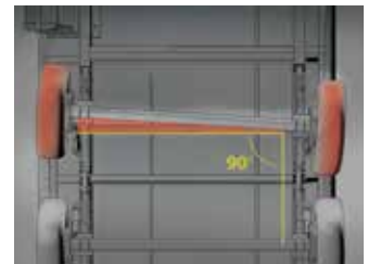
Misaligned suspension can cause uneven tire wear.
