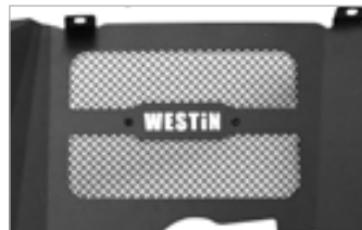
MESH COVERED OPENINGS TO PROVIDE ENGINE VENTILATION
