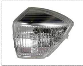
Mirror Side Blinker Unit WY5W
