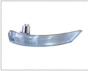
Mirror Side Blinker Unit WY5W
