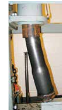
Competitor's 25K gooseneck fails longitudinal test at 11,500 lbs.
