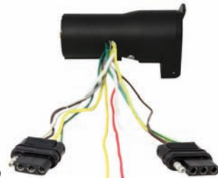
851010 7 Pin Universal Trailer Adapter • Plugs into most 7 pin trailer outlets • Two 4 wire flat connectors • 12v + and reverse leads for auxiliary lighting • Color coded wiring to match most trailer application
