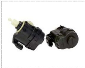
Leveling Motor 20-0797-MA-1 RH=LH 8200261818
