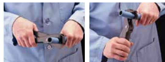
The rotating/rocking technique produces fast easy cuts.
