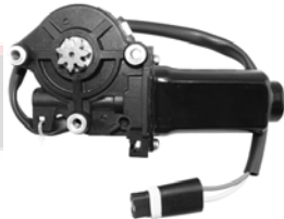
86806 A86806 ACI Plus Power Window Motor Chrysler (00-95); Dodge (02-94); Jeep (98-93); Plymouth (00-96) Chrysler: 4814118AB, 55154620, 56005164
