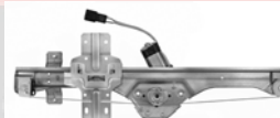
82315 F82315 ACI Plus Power Window Motor and Regulator Assembly Chevy (11-09); GMC (11-07); Saturn (10-07)
