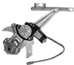
88156 D88156 ACI Plus Power Window Motor and Regulator Assembly Honda (01-97) Honda: 72751S10J01
