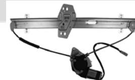
88535 D88535 ACI Plus Power Window Motor and Regulator Assembly Honda (08-03) Honda: 72710S9VA02
